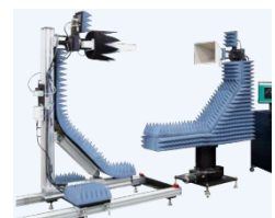
Antenna positioning and control system (0.5-20GHz, Antenna Size : Dia. 0.7m)
